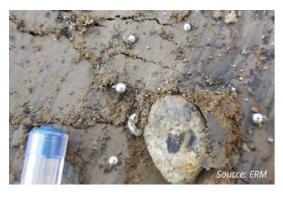
lemental Hg can collect in features such as subsurface drains, and the foundations, walls, floors and metallic structures surrounding industrial processes can incorporate Hg through adsorption. As a result, the selected site investigation techniques should be tailored to account for non-uniform contaminant distribution (so-called "nugget effect").
