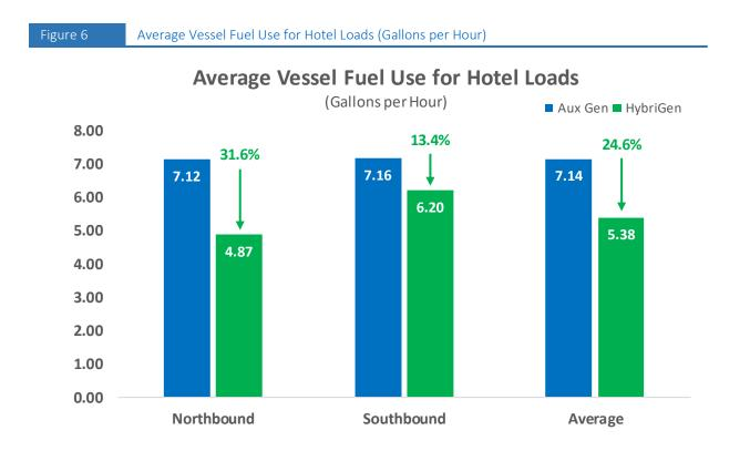
As shown, the HybriGen® Power system provided a fuel consumption benefit ranging from 13% to 32% for hotel power generation. Over the entire test period, the hybrid system averaged a 25% decrease in fuel use for hotel load.
