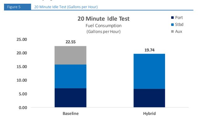
As shown, the HybriGen® Power system yielded a savings of 2.81 gallons per hour (~12.5% savings), when compared against both main engines and auxiliary generator set in the baseline condition. The power used to generate hotel load under the baseline condition is shown in gray, while under the hybrid condition, this hotel load is generated by the starboard main engine (light blue).
