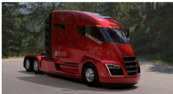
prosaically, perhaps, the Co-op chain of supermarkets in Switzerland has actually launched the world's first 34t fuel cell truck. Sweden's PowerCell provided the 100kW stack, integrated by SwissHydrogen and ESORO. The electric motor provides a steady 250kW and seven 700bar Luxfer tanks stacked behind the cab give the truck 32kg of usable hydrogen, and a range approaching 400km.
