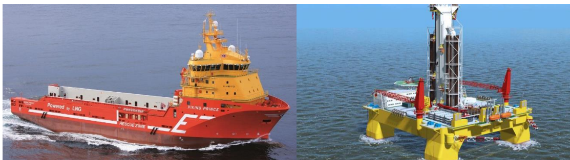
FIGURE 2 EXAMPLE OF SUPPORT VESSEL (LEFT) AND SEMI-SUBMERSIBLE DRILLING UNIT (RIGHT)
