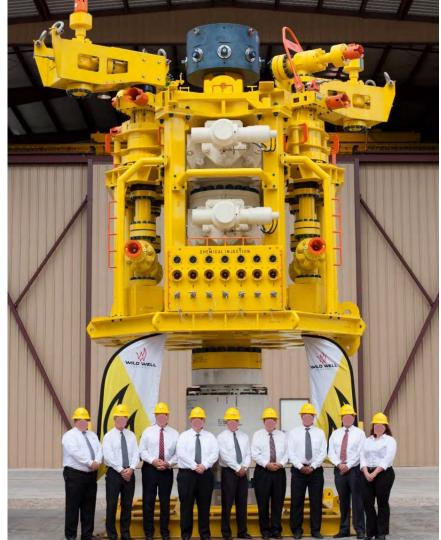
THE CAPPING STACK WILL BE MOBILISED FROM THE SHORE BASE IN THE VERY UNLIKELY EVENT OF BOP Source: ENI, 2018 FAILURE TO CLOSE, I.E A BLOWOUT EMERGENCY EVENT
