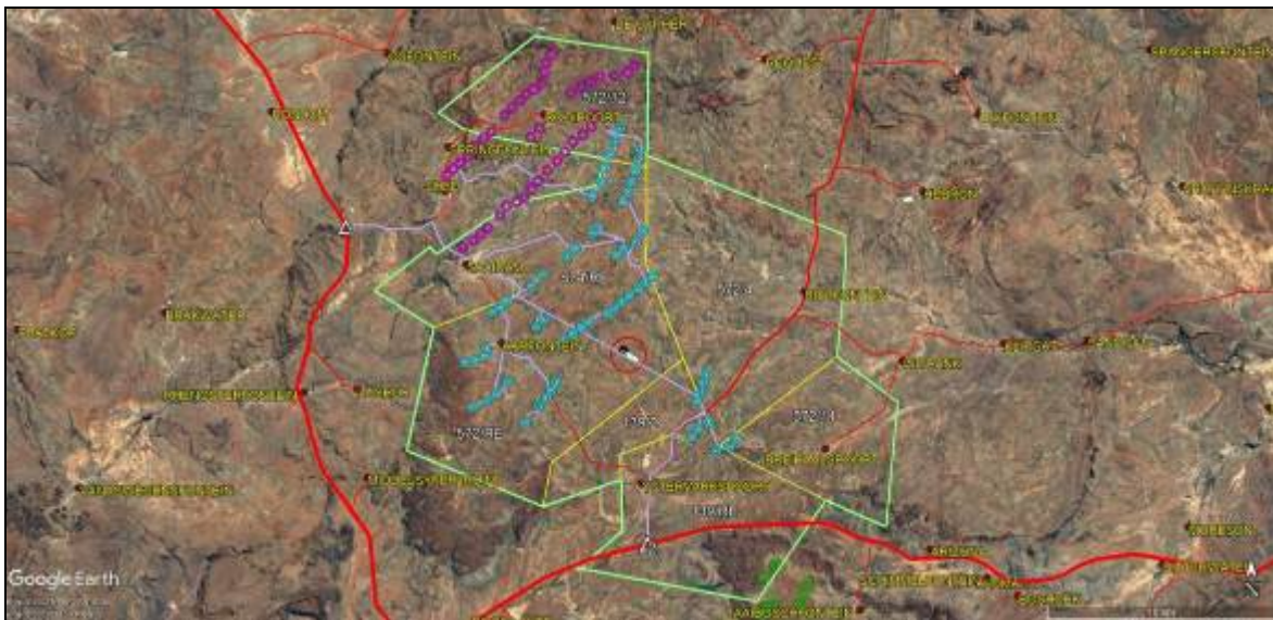
Figure 3.6: Loxton 2 WEF site properties (blue outline) in relation to proposed WEF 2 turbines (blue circles), construction- and operational phase terrain cluster (circled red), project roads (light purple), and site access Alts (white triangles). Also indicated are roads (red) and proposed Loxton 1 WEF (pink circles) and WEF 3 turbines (green circles).
