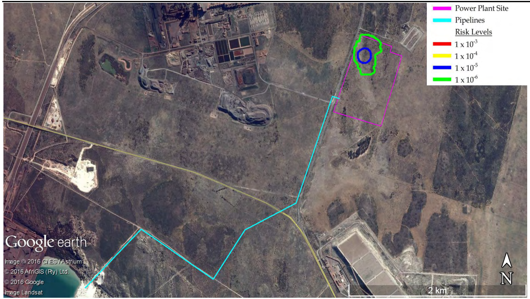
Figure 7.7 Risk Contours for Individual Risk of Fatality for Saldanha Steel Natural Gas Pipelines and Propane Developments during the Second Year of Construction – Persons Located Indoors
