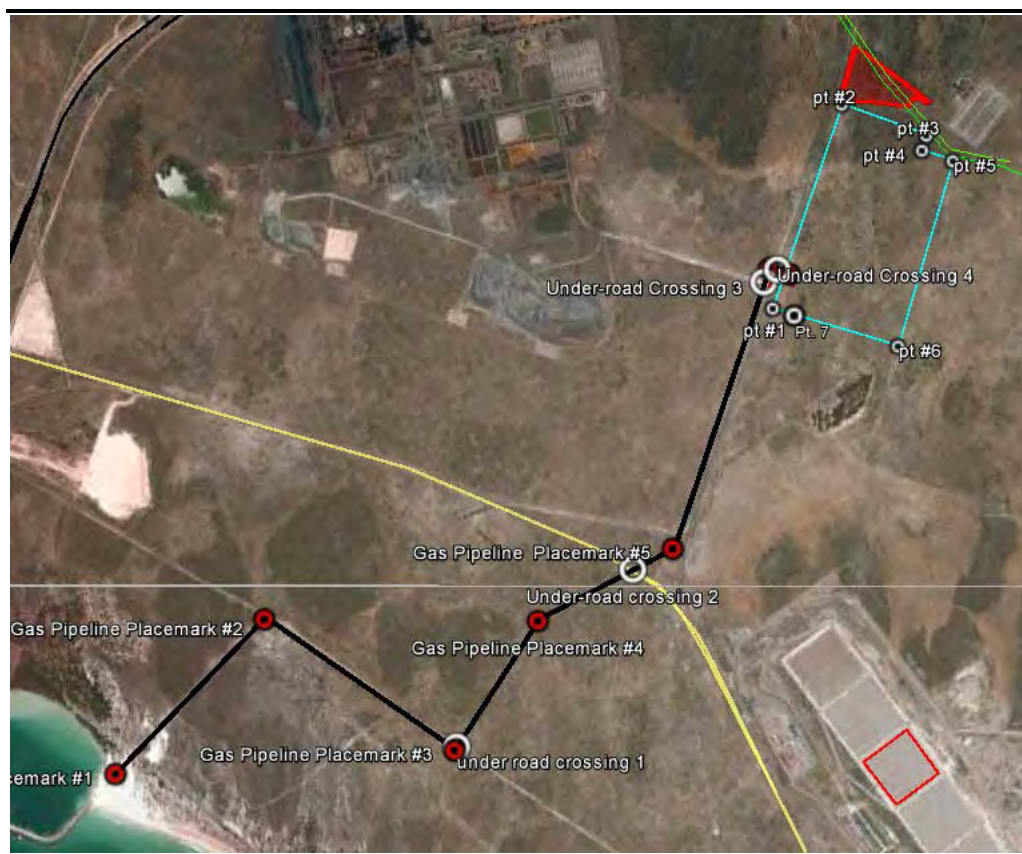
Figure 1.1 A Map of the Proposed Natural Gas Pipelines to the Proposed CCGT Power Plant
