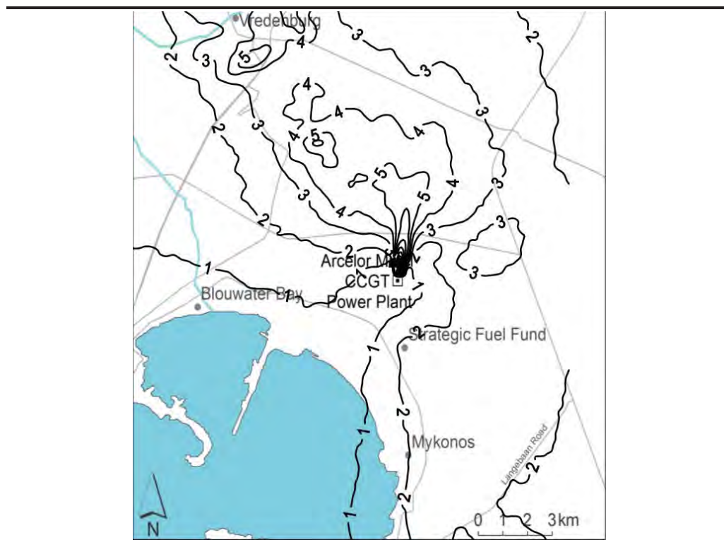
Figure 10.4 99th percentile of the predicted 1-hour CO concentrations ( \mu\text{g}/\text{m}^3 ) resulting from emissions from ArcelorMittal CCGT power plant (operation)
