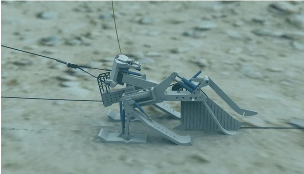
Figure 2-20 Animation of Cable Burial Plough on Seabed
