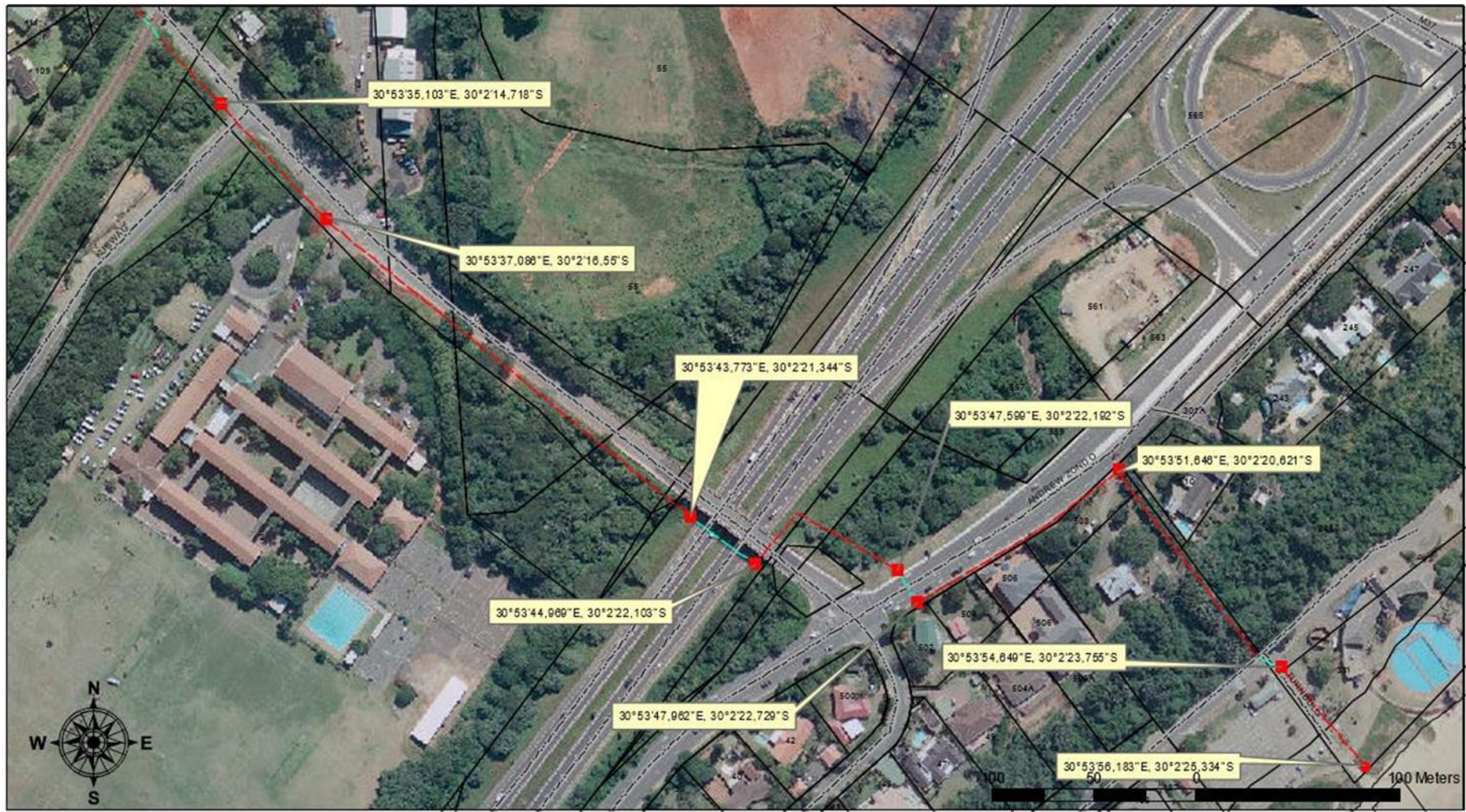
Figure 3-2 Section of the Terrestrial Cable Route 1
