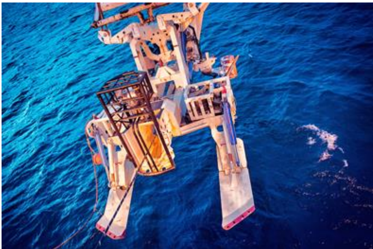
Figure 2-19 Elettra – Taurus 2 SMD Plough System
