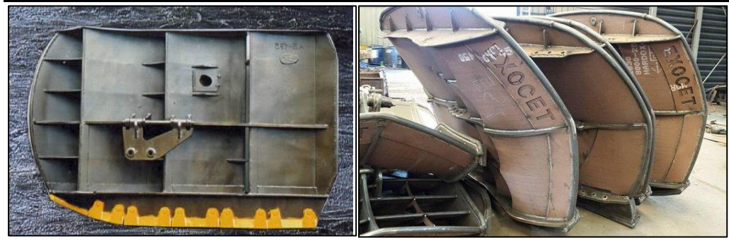
Figure 9.4 Photographs of trawl doors typically used as part of ground gear in the South African demersal trawl fleet.
