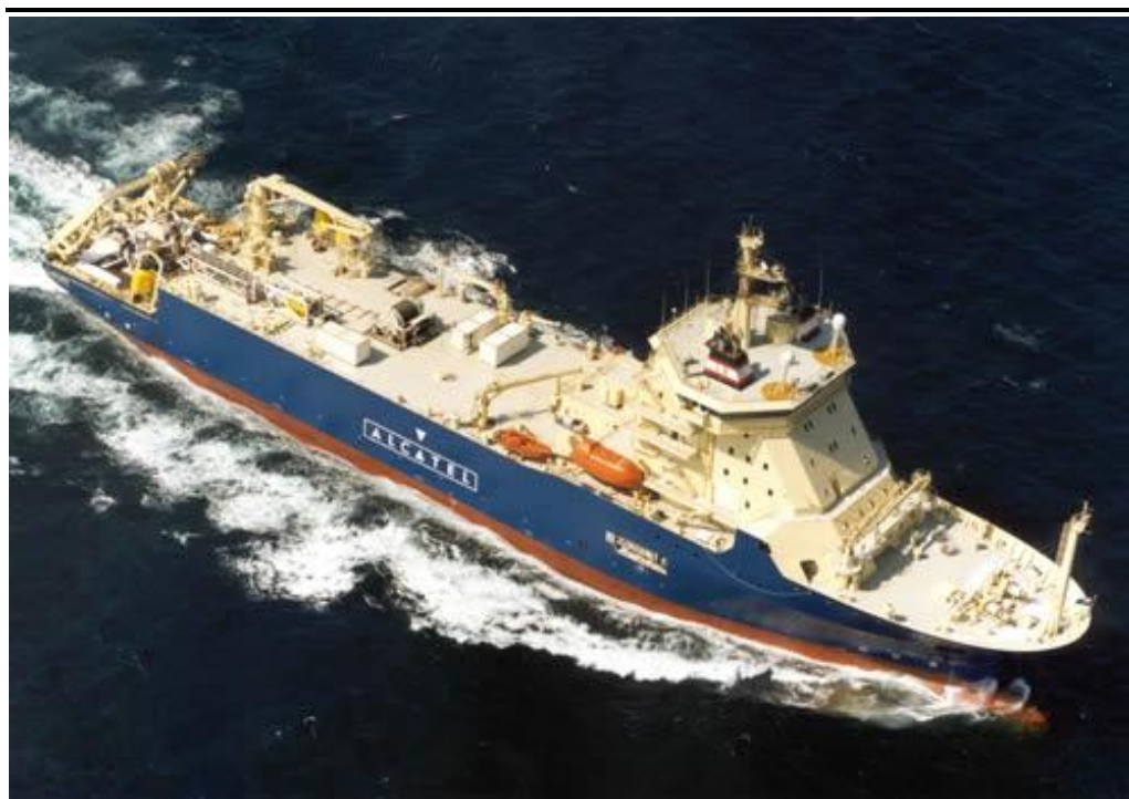
Figure 2.6 Typical Cable Laying Ship
