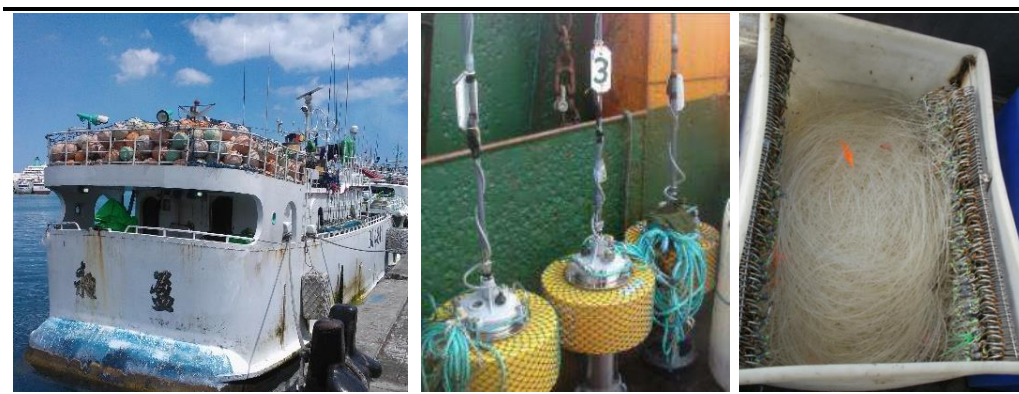
Figure 5.9 Photographs showing marker buoys (left), radio buoys (centre) and monofilament branch lines (right)
