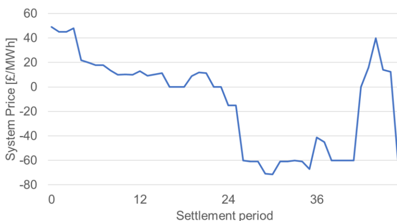
Figure 5: System Price of electricity in GB in the 48 half hourly settlement periods on 26/05/2019
