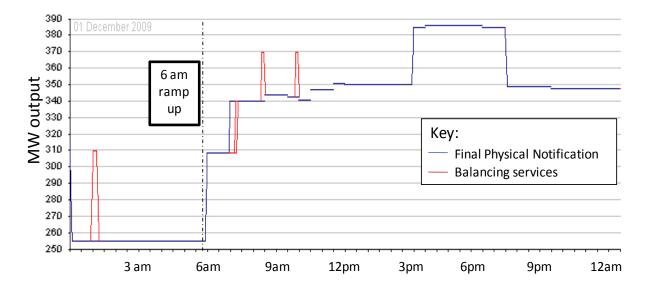
Figure 38 Example output of a gas power station module across 1 day, including the final expected output (FPN) in the absence of the balancing mechanism and output including balancing services required (shown in red).
