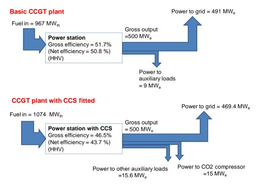
Fuel requirement x CO<sub>2</sub> intensity of fuel x (1-% emissions captured) = CO<sub>2</sub> emitted
