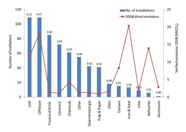
Note: figures shown above columns indicate average sector direct  $CO_2$  emissions per installation in  $MtCO_2/yr$ Source: UK Phase II NAP data (sector data includes CHP emissions)
