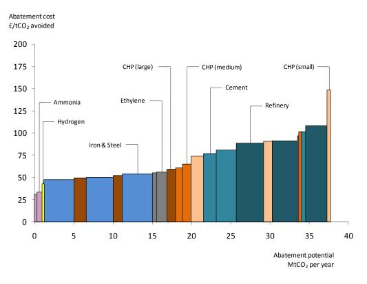
The lowest cost options for industry CCS consist of, in order of abatement potential: iron and steel blast furnaces, larger CHP facilities, and high purity  $CO_2$  streams such as those produced from ammonia and hydrogen production plants. These can deliver the first 15Mt of  $CO_2$  abatement below or around £50/tCO<sub>2</sub> abated.
