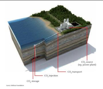
Figure 1 Idealised power station with capture, transport and storage (Image courtesy The Bellona Foundation).
