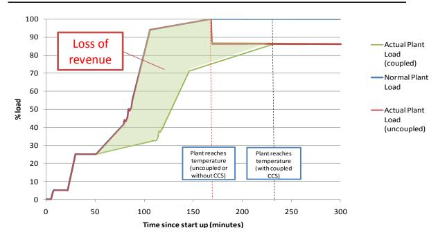
Figure 40 Cold start-up post-combustion capture plant with and without coupling.
