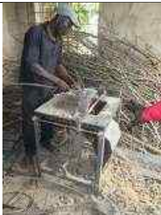
Preparation of feedstock using circular saw
