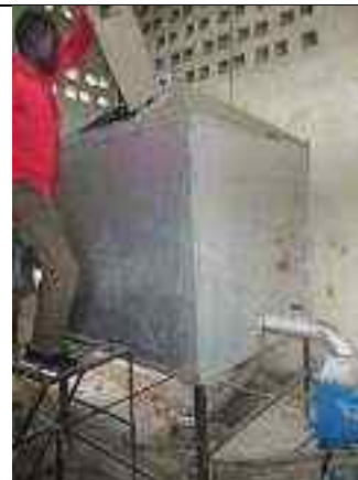
Wood dryer (heated from engine exhaust)
