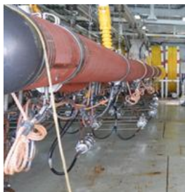
Figure 1.2: Airguns on-board a seismic vessel prior to deployment. These are the sound sources that develop the signals directed to the sea-floor.
