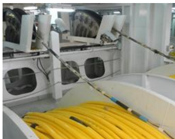
Figure 1.3: A typical streamer containing hydrophones ready to be deployed. These are towed behind the seismic vessel to record returning sound signals.
