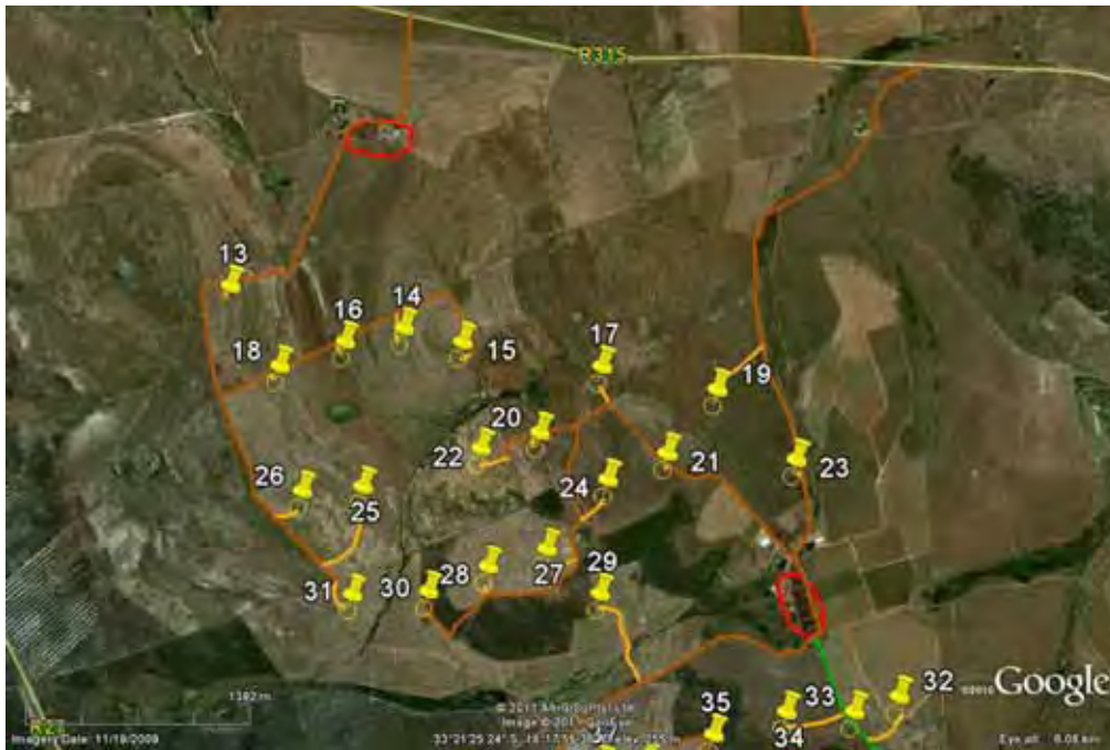
Figure 2: Proposed Alternative 2 layout in central area. Roads and cable trenches are assumed to be closely parallel, and are indicated in brown, green and yellow. The red balloon is the primary laydown area.
