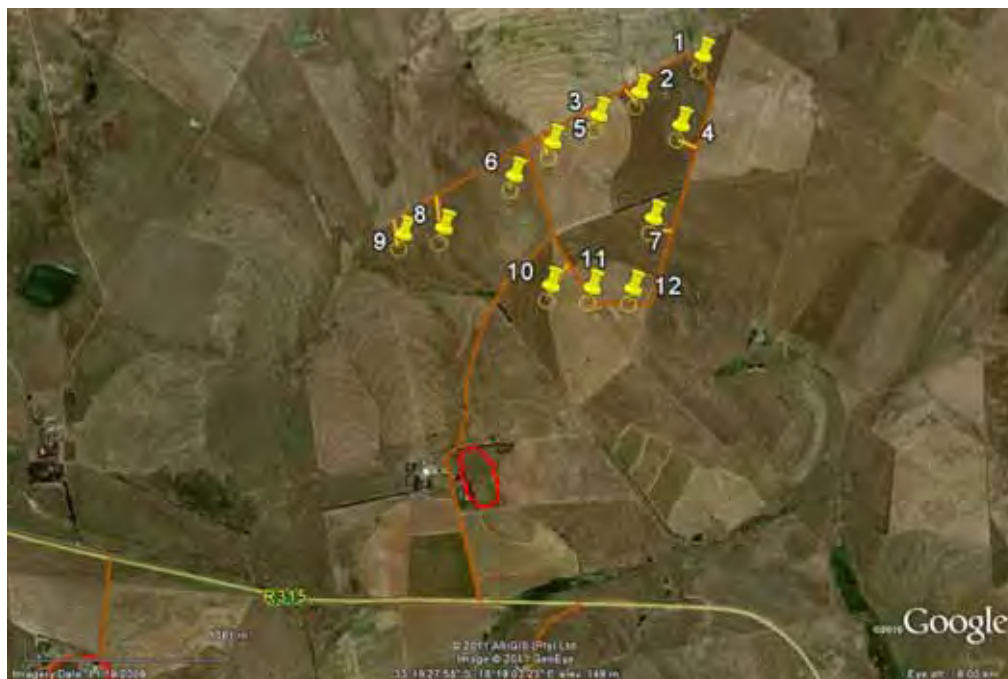
Figure 1: Proposed Alternative 2 layout in northern area. Roads and cable trenches are assumed to be closely parallel, and are indicated in brown and yellow. The red balloon is the primary laydown area.
