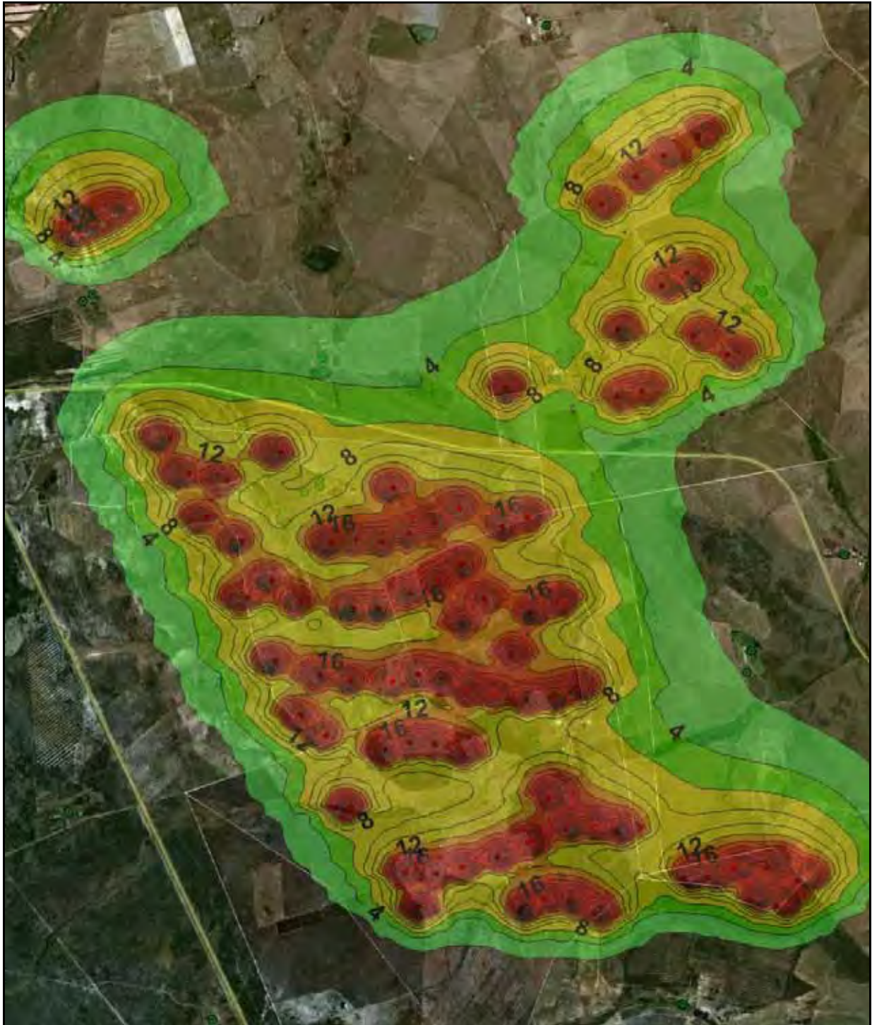
Figure 7-10: Operational Phase: Change in ambient sound levels, contours of constant noise levels with a southern wind blowing at 5 m/s
