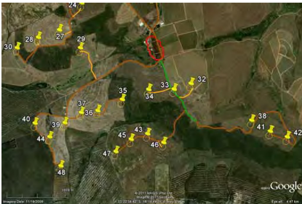
Figure 3: Proposed Alternative 2 layout in southern area. Roads and cable trenches are assumed to be closely parallel, and are indicated in brown, green and yellow. The red balloon is the primary laydown area.
