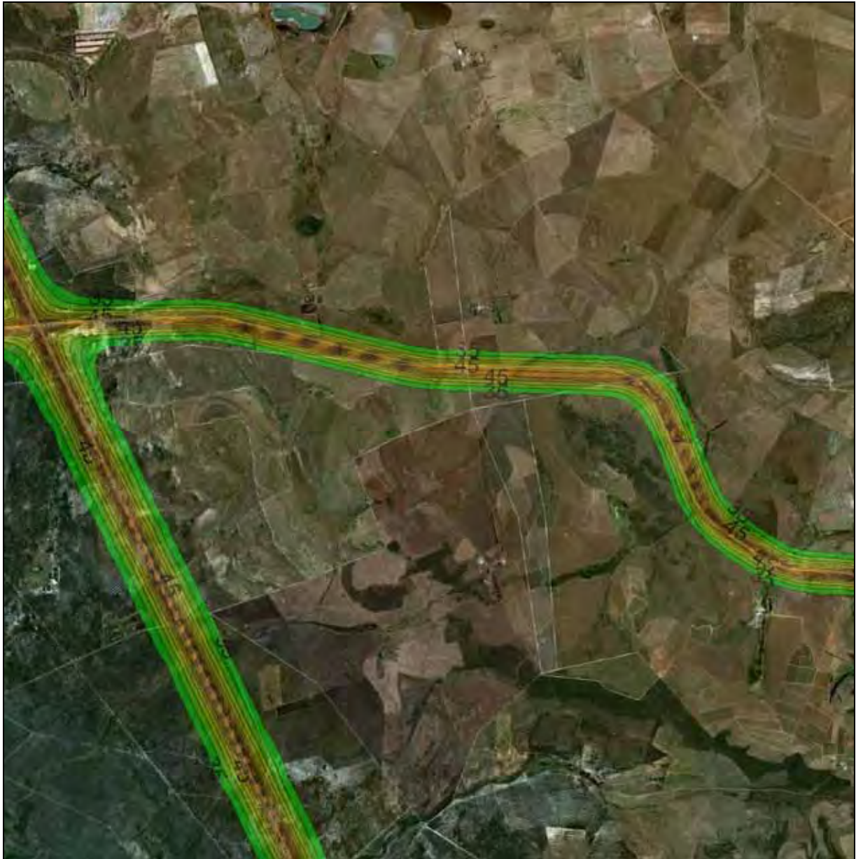
Figure 3-3: Daytime (06:00 – 22:00) ambient sound levels: Contours of constant sound levels
