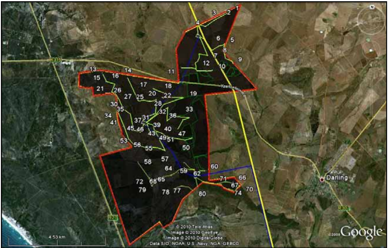
Figure 82: Aerial view of the proposed WEF area showing the overhead power line in dark blue. The yellow line running north-south is an existing power line whose course would be followed up to the Dassenburg substation.
