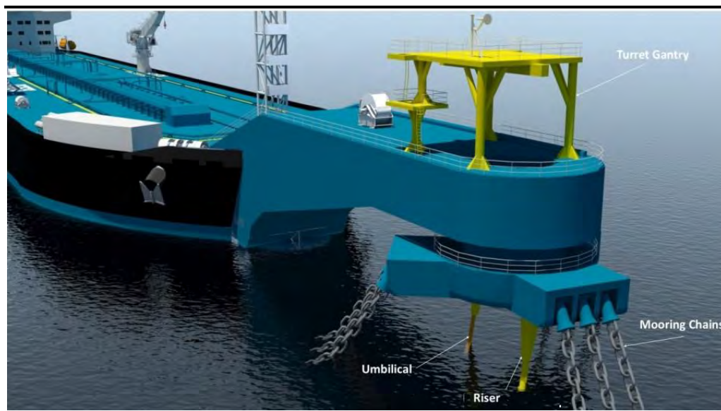
Figure 2.10 Turret Mooring System (TMS)
