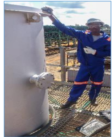
Measuring emissions from the plant stacks as a basis for air pollution modelling of cumulative impacts.
