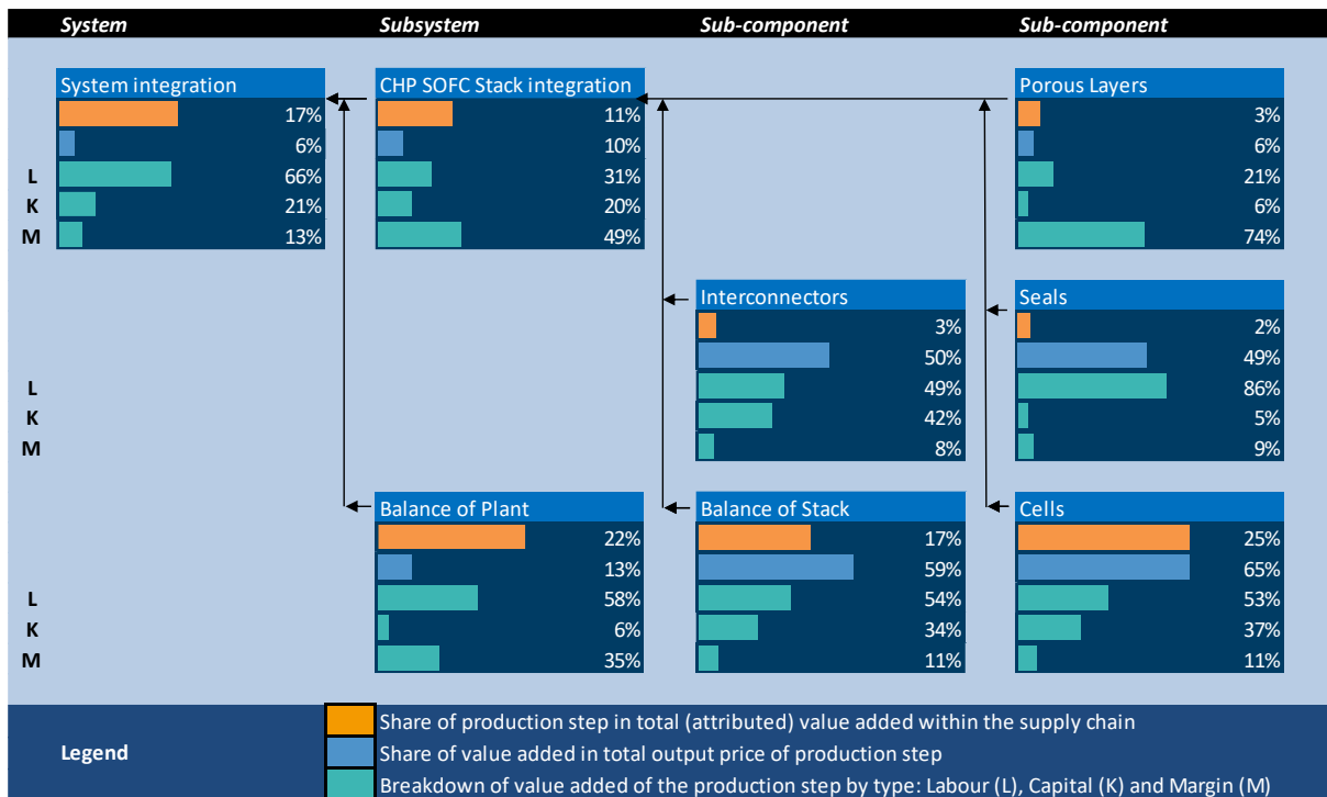
Figure 44: Value-added decomposition for FC system for SOFC CHPs, low market deployment scenario, 2030
