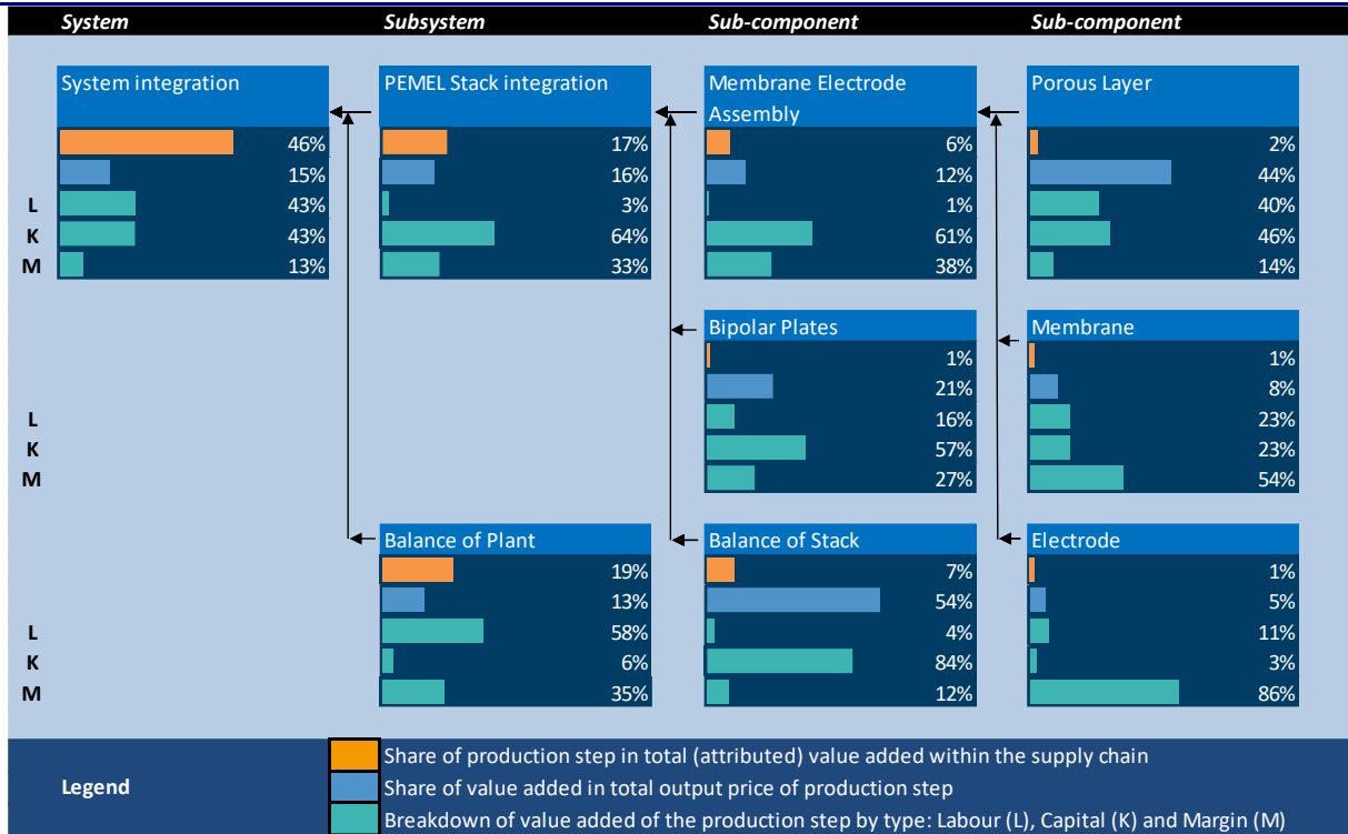
Figure 41: Value-added decomposition for PEM electrolyser systems, high market deployment scenario, 2030
